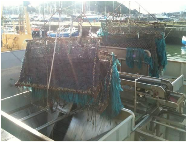
Figure 2. Mussel dredges. Photo: Kat Collinson, MEP
