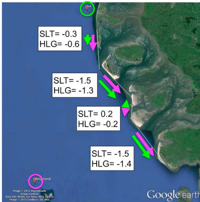
Figure 2.17 Littoral drift along the Schleswig Holstein coastline, computed using wave data from stations Helgoland (HLG, magenta arrows) and Sylt (SLT, green arrows), in 10^6 \text{ m}^3/\text{yr} (From: Ridderinkhof, 2016).
